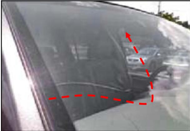
Single crack with **no** impact mark:
