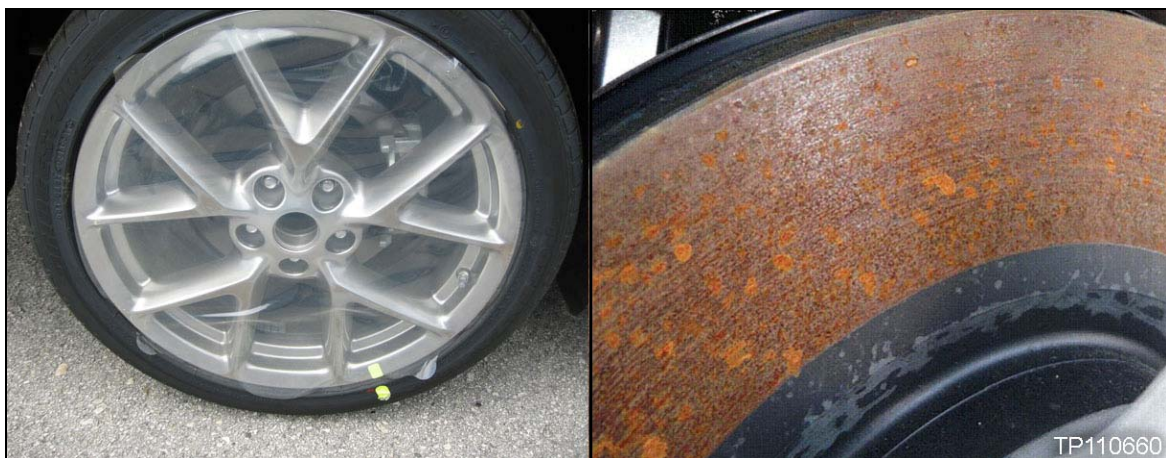
Wheel protector covers help prevent cosmetic rotor corrosion.
